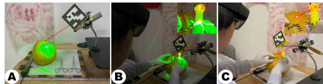
Fig. 5: The LPA-assisted puncture process involves the following steps. First, the operator anchored the virtual path (A and B). Then, the crosshair laser was turned off, and the puncture was performed from a lateral perspective with axial locking (C).
